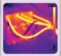
Energy losses from mould temperature controller piping can be considerable
